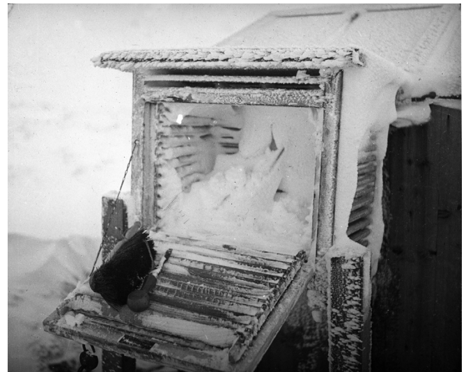
Fig. 8. Stevenson screen full of snow and ice, n.d., GB 033 MAN 8/135, Durham University Library, Archives and Special Collections.
