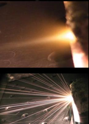
Laser ablation resulted in the formation of a gaseous plume of ejecta; similar to the development of a rocket exhaust. A comparable ablated mass flow rate between the experiment & the theoretical model was also observed. However, the ejecta did include some solid particles. This will enhance the transfer of momentum, and is not currently accounted for in the numerical model. The degrading affects of the deposited ejecta were also considerable different.
