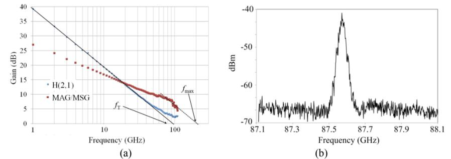
Figure 2. The current gain and the maximum available gain/maximum stable gain versus frequency for a two-finger pHEMT with 12  $\mu\text{m}$  width (a) and the measured spectrum of the 60  $\mu\text{m}$  wide Gunn diode with 1.3  $\mu\text{m}$  anode to cathode separation (b).
