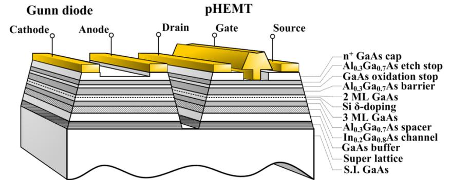
Figure 1. The layer structure and the implementation of the two devices on the same substrate.
