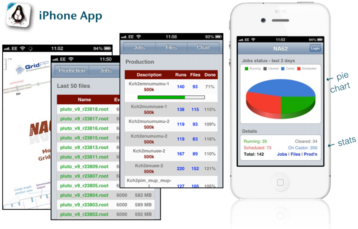
FIG. 8: Annotated screenshots of the NA62 iPhone WebApp for Grid production monitoring. To install this app on your smartphone, navigate to http://na62.gla.ac.uk/app/ and use the 'Add to Home Screen' option.
