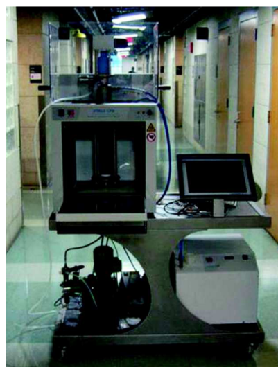
Figure 4. Milestone Flowsynth continuous-flow MW reactor. 42 Reprinted with permission from ref 42. Copyright 2008 American Chemical Society.
