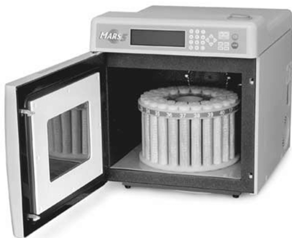
Figure 3. CEM MARS multimode MW reactor. Copyright 2003. Reprinted from ref 38 with kind permission from Springer Science and Business Media.
