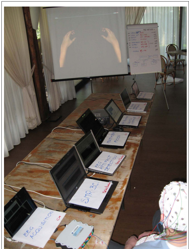
FIGURE 7 | This picture was taken during the demonstration of the proof of concept. Here, all connected computers, forming a demo hybrid BCI, are visible. The first was used for data acquisition, running the SignalServer, and the next two were used to build an SMR BCI and an artifact detection. Laptop number four was a very simple implementation of fusion. Laptops five and seven formed together the visual feedback, presented on the screen (control interface and feedback application). The sixth laptop showed an additional operator feedback which was not presented to the subject.
