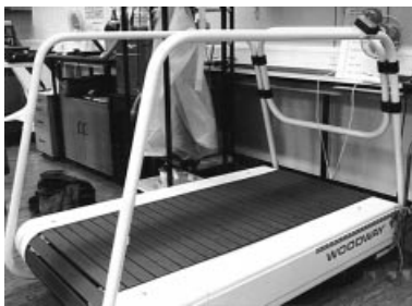
Figure 2 The 'Woodway' treadmill. The slatted construction of the running surface is apparent.
