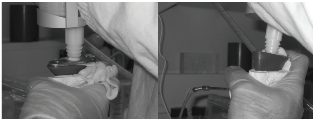
Figure 3 During the pressurisation the cement leaked more around the conventional pressuriser (left) compared to the modified pressuriser (right).
