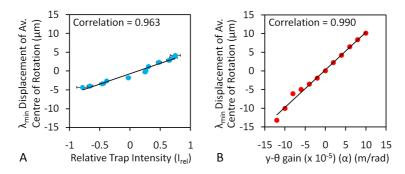
Fig. 3. Control of the location of the average centre of rotation along the length of the probe, with the traps placed  $12 \,\mu m$  apart. (a) Control by varying the relative intensity of the trapping beams. (b) Control by variation of the y- $\theta$  term in the gain matrix enabling the centre of rotation to be moved outside the region between the two traps.
