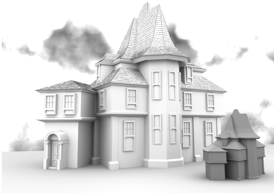
Figure 1: Procedural extrusions allow a footprint (2d plan) to be extruded to form the walls and roof of a house (inset). Meshes and procedural details can then be attached (main).
