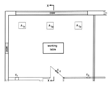
Figure 1 Plan view of cleanroom,  $A_t$  = air inlet, E = exhaust grilles, DGW = double glazing window
