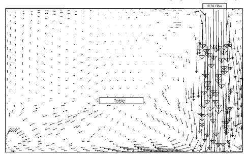
Figure 9 CFD simulation of the air flow in a cleanroom with 15 air changes per hour and an air jet from supply inlet
