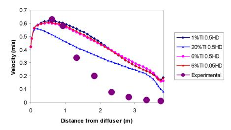
Figure 7 Effect of turbulent intensity and hydraulic diameter on the air throw from a 4-way diffuser
