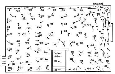
Figure 3 Airflow from a 4-way diffuser
