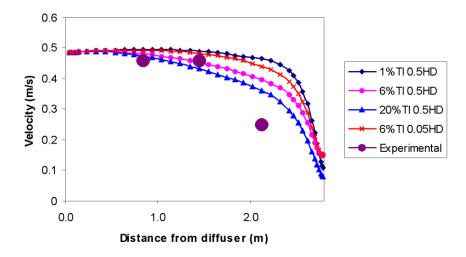
Figure 6 Effect of turbulent intensity and hydraulic diameter on the air throw from an inlet without a diffuser
