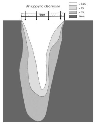
Figure 5 Penetration of particles from the cleanroom into a air jet from an inlet with no diffuser
