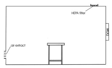
Figure 2 View of cleanroom at section X-X. DGW = double glazed window.
