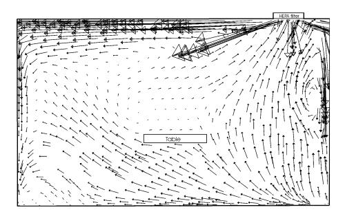
Figure 8 CFD simulation of the air flow field in a cleanroom with 15 air changes per hour and a 4-way diffuser
