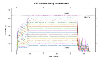
Fig. 3. CPU load over time for different connection rates.
