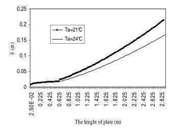
Fig 5: Boundary layer thickness of the full developed air flow at  $T_P = 90$ °C.
