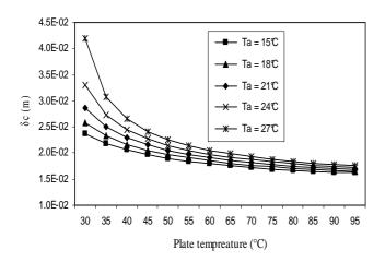
Fig 4: Thickness of the boundary layer at the critical height for different plate temperatures.
