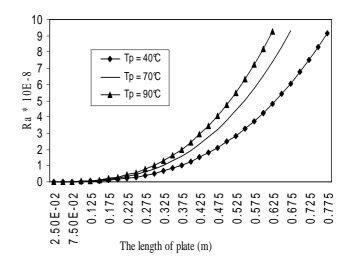
Fig 1: Rayleigh number at different location on the vertical plate at  $T_a$  =25°C.
