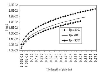
Fig 2: Thickness of the boundary layer along the vertical plate at  $T_a$  =25°C.
