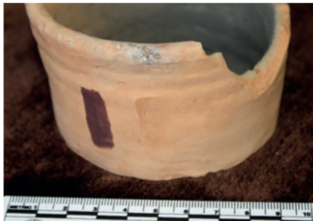
Figure 13.3.4 (Modern) pot made of Orcadian clay showing painted decoration using haematite (left band) and iron-rich sandstone (right band) after firing at 500°C for 3 hours.
