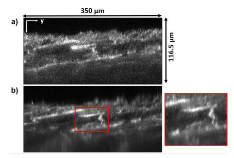
Figure 4. Fluovolt stained ventricular slice imaged by a) conventionally translating the sample objective and b) remote refocusing z-y frame scanned at 122 Hz axially. Qualitatively the structures are comparable and cell demarcations (highlighted red) are clearly visible.
