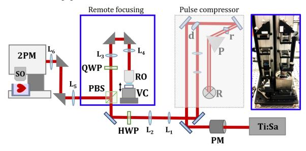
Figure 1. Experimental set up with an ultrafast laser as excitation source for a commercial 2-photon microscope with custom-built remote focusing and pulse compression units. QWP, HWP: quarter- and half-wave plates. PBS: polarizing beam splitter. VC: voice coil actuator. PM: power modulation. RO: remote objective. SO: sample objective. d, r: d-shaped and roof mirrors, respectively. P: prism, R: retroreflector. The arrow indicates the direction of remote mirror actuation.
