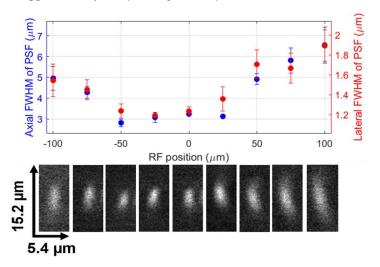
Figure 3. RF-2PM system resolution across the dynamic range of refocusing.
