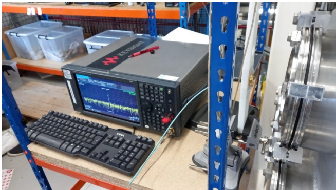
Figure 2: Rx side spectrum analyzer with WR-22 transition held outside a DN200 ISO-K port on right.
