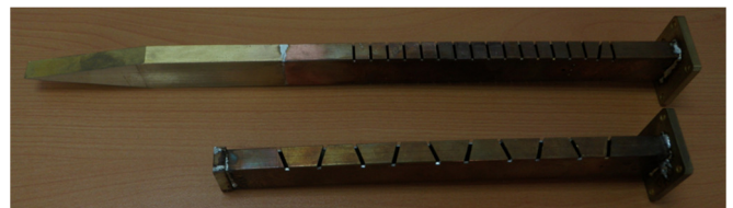
Figure 1: Photograph of a copy of Watson's Yagi antenna with 10-slot antenna for scale comparison.
