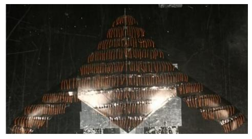
Figure 12. Tufts stuck onto the model surface.
