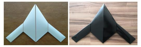
Figure 8. 3D-printed model (left) and surface finished and painted model (right).
