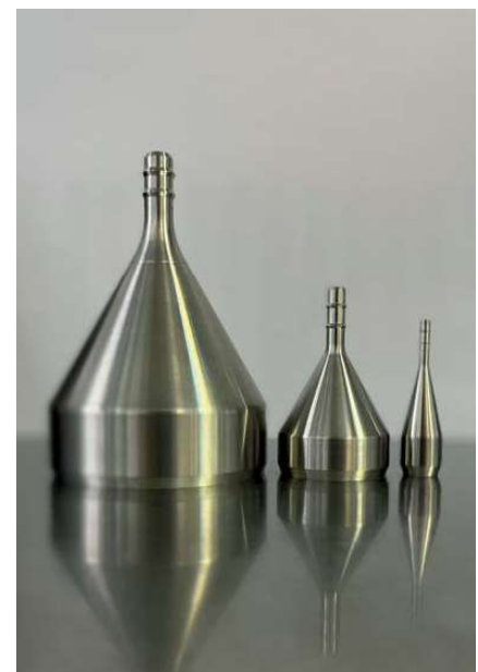
Figure 2: Isokinetic probes for sampling 2.8, 28, and 100 L/min of air (normally turned to face unidirectional airflow)
