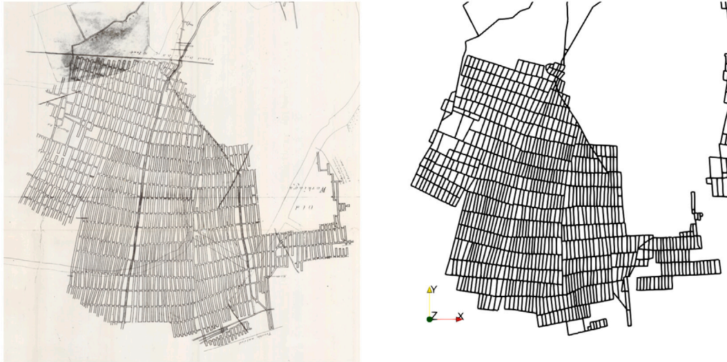
Fig. 1. Left hand side showing an original mine plan from the UK's Coal Authority. The dimensions are about 500 by 500 m. The right hand side shows the result of the digitisation of the mine plan using GIS.
