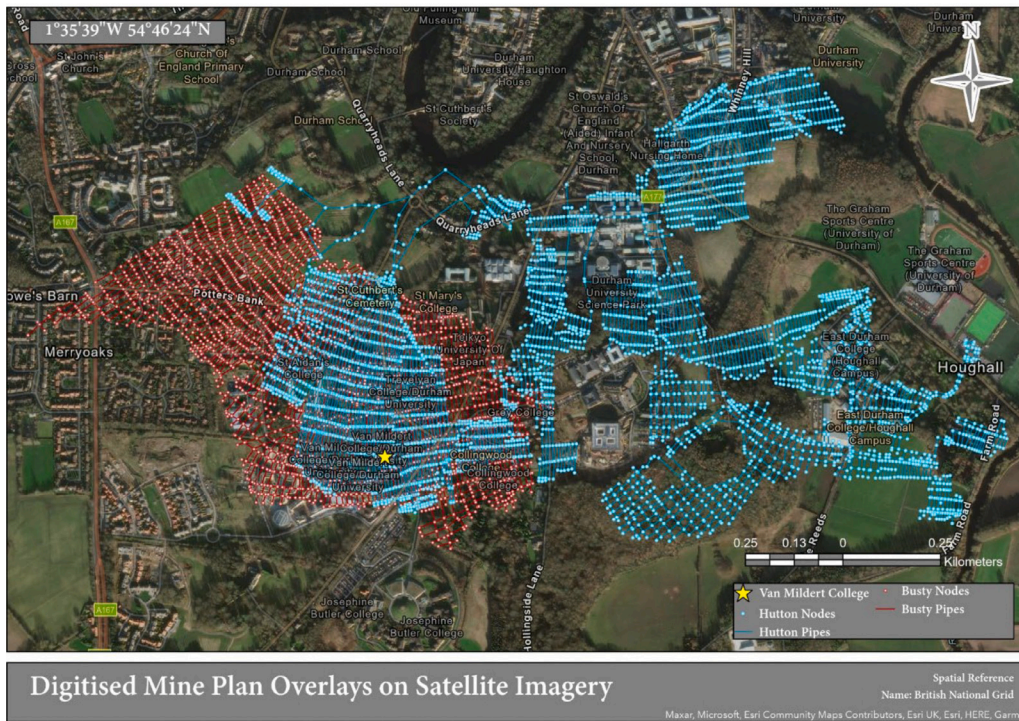
Fig. 3. Digitised mine plans showing the Busty Seam in red, the Hutton Seam in blue. The yellow star indicates the location of the Van Mildert College of Durham University. Source: From [40].
