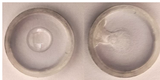
FIG. 4. Reaction of titanium(IV) propoxide liquid with moisture from the air. On the left: titanium(IV) propoxide under dry air conditions; on the right: a droplet of titanium(IV) propoxide after 5 min of exposure to natural air, both contained in a 17 mm diameter glass crucible. Note that the humid air exposed sample has turned to chalky white, indicating the formation of \text{TiO}_2 and loss of the original liquid structure.
