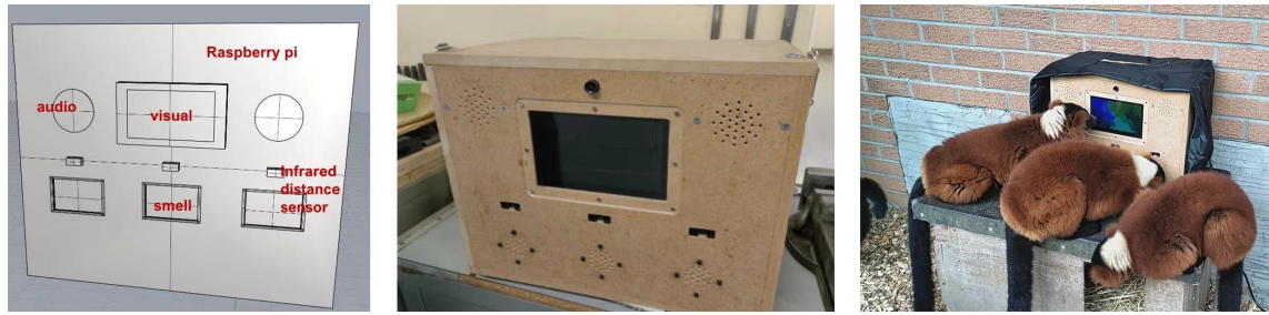
Fig. 1. Left: Drawings of the device. Centre: Sensory stimuli device. Right: Image of the lemur engaging with the device.
