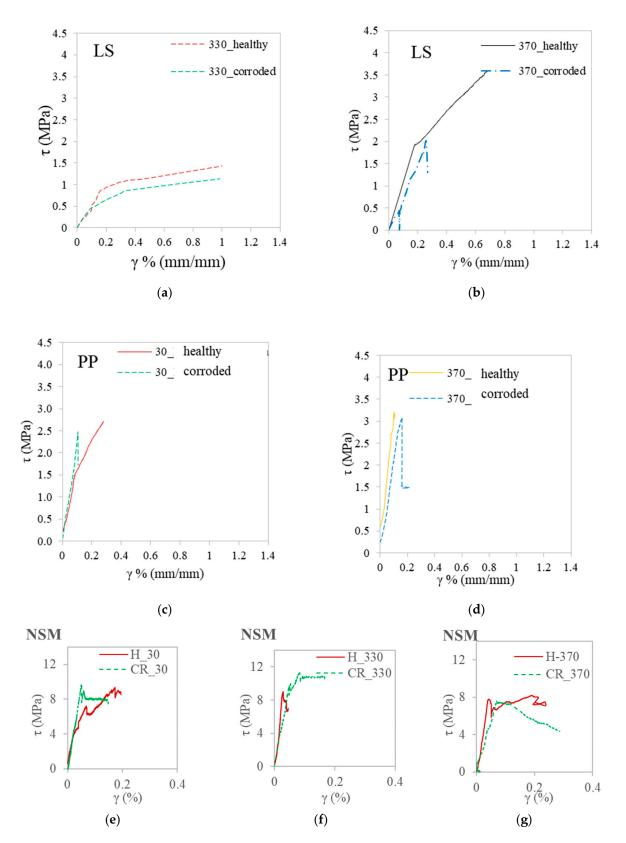
**Figure 8.** Mean curves of shear stress-strain experimental results for prisms of healthy or corroded substrate externally bonded with laminated sheets-LS: (**a**) standard epoxy and (**b**) toughened adhesive, with prefabricated plates-PP: (**c**) standard adhesive and (**d**) toughened adhesive and containing NSM bars (**e**,**f**) standard adhesives and (**g**) toughened adhesive.
