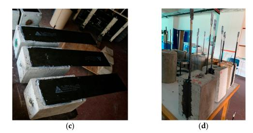
**Figure 5.** Application of FRPs and curing: (a) applying primer and application of the fabric, (b) impregnation of epoxy layer following the fibers' direction, (c) prefabricated plates, and (d) NSM integration.
