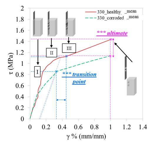
Figure 7. Mean shear stress-strain experimental curves for specimens with laminated sheets.
