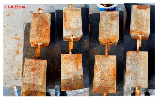
Figure 3. Corroded substrates: crack pattern and opening range.
