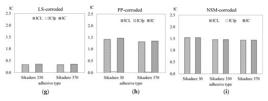
**Figure 9.** Interface Capacity (IC) indices vs adhesive type bar chart: (**a**,**d**,**g**) laminate sheets-LS, (**b**,**e**,**h**) prefabricated plates (PP) and NSM (**c**,**f**,**i**).
