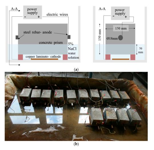
Figure 2. Accelerated corrosion (a) schematic map and (b) curing specimens in the tank (wet conditions).
