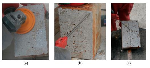
**Figure 4.** Interface treatment: (**a**) smoothing the surface using a grinding wheel with diamond cutters (**b**) surface and (**c**) crack cleaning by high-pressured air.
