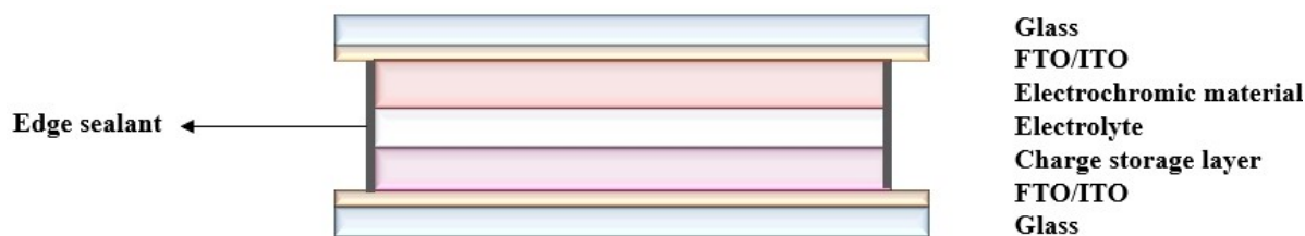
Figure 1. Major components of an ECD (Adapted from reference). [16]
