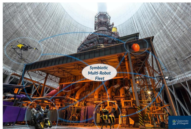
FIGURE 15 Composite image of a SMuRF in an industrial environment highlighting infrastructural sensors, ground and aerial vehicles positioned together.
