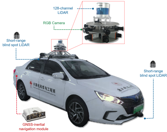
Fig. 5. Configuration of the testing vehicle for the real-world road test, equipped with a 128-channel LiDAR, a high-precision GNSS-inertial navigation system, and an onboard computer for hosting the software.
