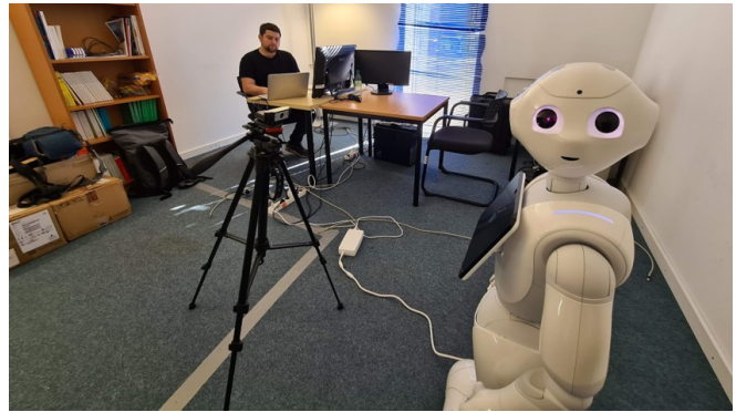
Fig. 1. The lab settings, including the robot Pepper in front of a web camera, while the experimenter in the back is controlling the robot using the Wizard-of-Oz technique.
