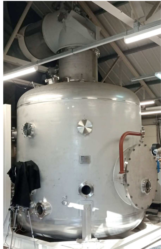
FIG. 1. Test chamber of the plume-regolith test facility.
