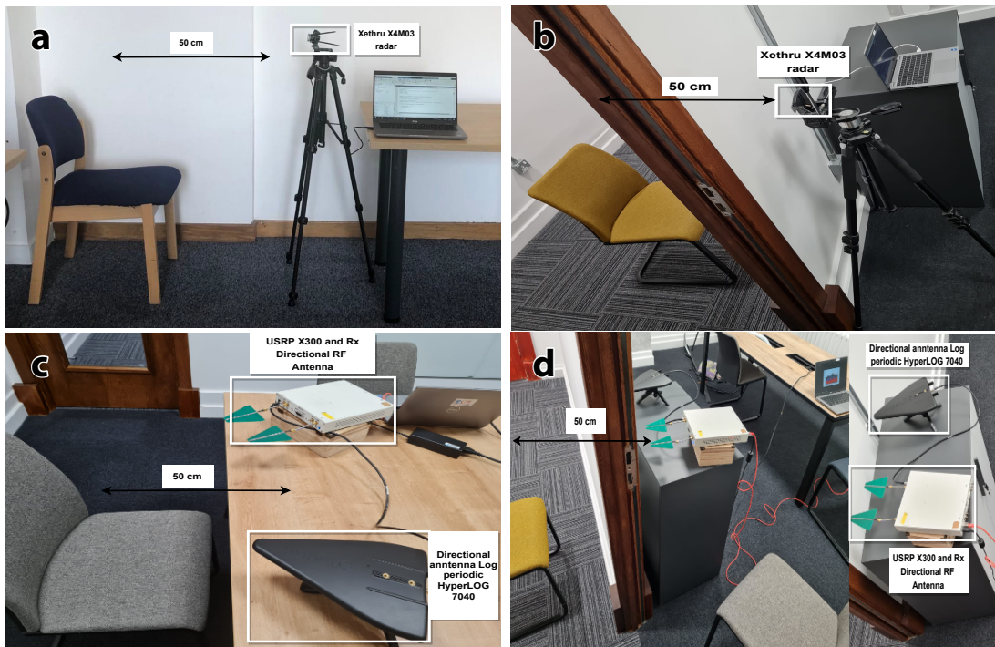
Fig. 3. Head movements activity with their representation in Wi-Fi and radar signal. (a) An experimental setup of the radar signal without a wall. (b) An experimental setup of radar signal through a wall. (c) An experimental setup of Wi-Fi signal without wall. (d) An experimental setup of Wi-Fi signal through a wall.
