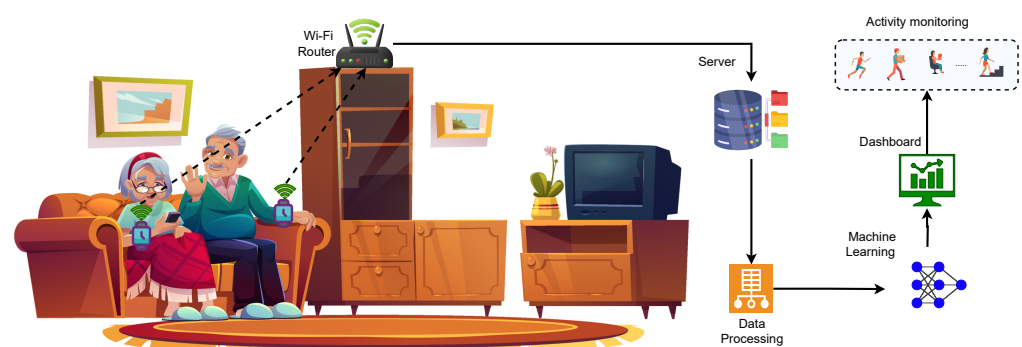
Figure 1. Conceptual framework of centralised indoor HAR using wearable sensors
