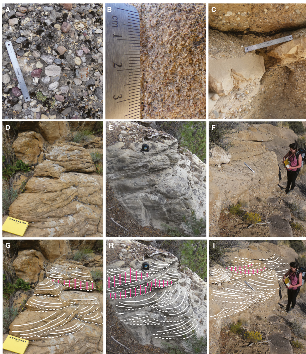
Fig. 4. Field data collection included grain-size measurements for (A) gravel and (B) sand fractions, as well as (C) estimates of the proportions of different grain-size facies. Parts (D) to (F) depict cross-bedding, and parts (G) to (I) depict interpreted versions of the same images. Dashed white lines indicate bounding surfaces of individual cross-sets and solid white lines indicate selected foresets within individual cross-sets. To exemplify sampling procedure when determining mean cross-set height, solid pink lines demonstrate how heights are measured for selected cross-set dip sections. Field notebook with 15 cm scale, tape measure and 30 cm rule for scale.
