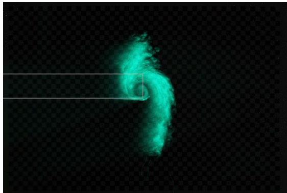
Figure 12. Final vortex image superimposed with grid paper and wing profile.
