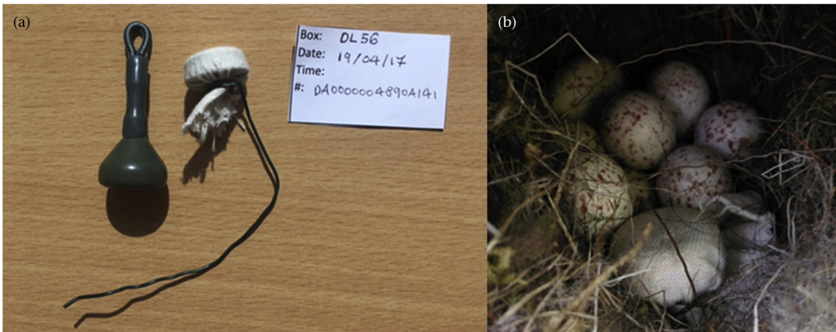
Figure A1. iButton set-up for incubation data collection. (a) Preprogrammed iButton wrapped in fabric and attached to wire (weight 28.35 g) and iButton field label. (b) Detail of a nest cup with the iButton device positioned among great tit eggs.
