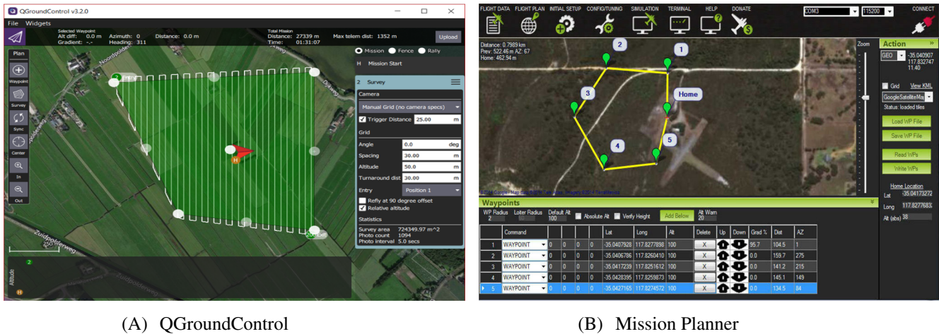
FIGURE 1 Illustration of the path-planning tools in (A) QGroundControl and (B) Mission Planner.
