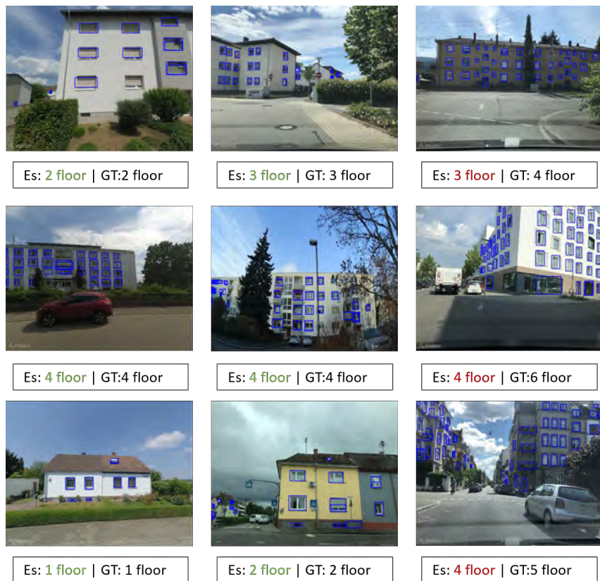
■ Figure 4 Selected examples of facade object detection and floor number estimating from Mapillary images in Heidelberg.
