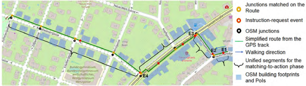
■ Figure 1 Preprocessing steps applied to the GPS tracks: smoothing (green line), OSM junction extraction and mapping to the route (black and yellow circles), instruction-event alignment (red circles), segmentation into unified segments with class labels (E1–E4), and extraction of land use and POI information from OSM in a 30m buffer around the route.
