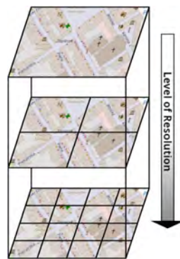
■ Figure 1 From top to bottom: The initial map is divided progressively into equal parts, thus creating a quadtree with different resolution levels.
