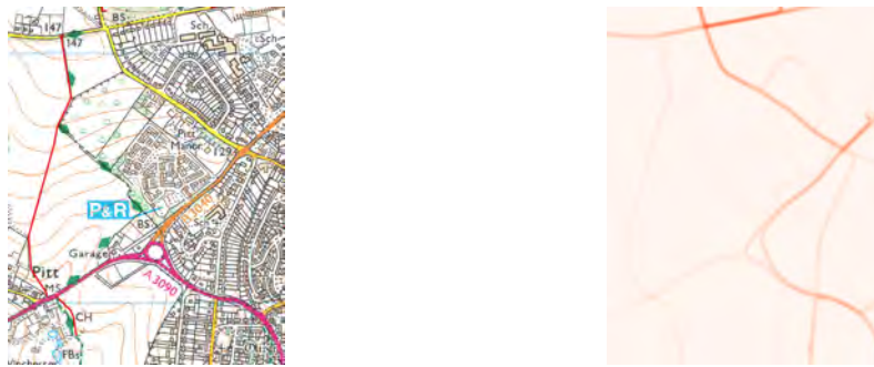
(a) New path shown in red, existing legal right of way shown as green diamonds. (b) line density raster with line intensity indicating relative level of use of the two paths.
