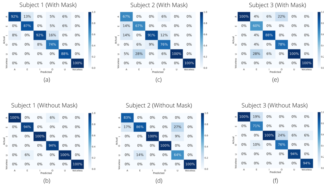
Fig. 5: ResNet50 model outcome in terms of confusion matrix of (a) subject 1 male with mask scenario (b) subject 1 male without mask scenario (c) subject 2 female with mask scenario (d) subject 2 female without mask scenario (e) subject 3 female with mask scenario (f) subject 3 female without mask scenario.
