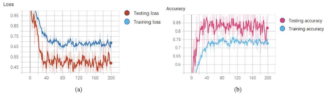
FIGURE 15 Loss curve and accuracy curve when the learning rate is 10^{-4} . The shaded curves represent the raw data and the trend lines are calculated using an exponential moving average. (a) Loss epoch. (b) Accuracy epoch.
