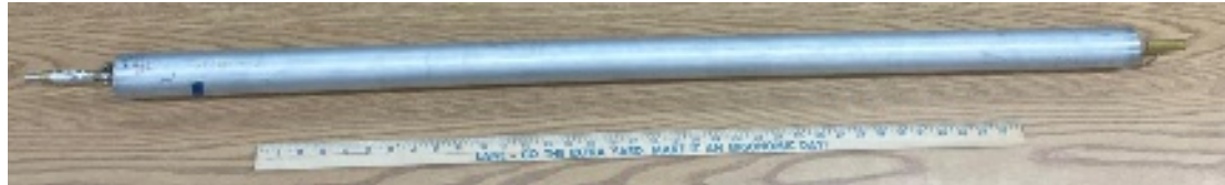
Figure 3. Laboratory Test Drift Tube. The GMT consists of drift tubes similar to the pictured test drift tube. Differences are length (1.8 or 2.4m in the GMT), and end connections for compatibility with GMT sockets.
