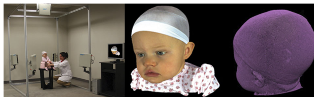
Fig. 2 Left: 3dMD's static 5-viewpoint 3dMDhead system was used to capture the Headspace dataset. Each of the 5 viewpoints is a 3D camera system that has an IR projector, IR camera and RGB camera. The system stitches the 5 point clouds into a single 3D output mesh, and provides the texture coordinates for texture mapping. Centre: texture mapped output mesh. Right: 3D point cloud output
