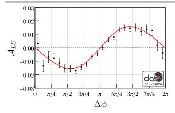
FIG. 2. The beam spin asymmetry  $A_{LU}$  as a function of  $\Delta \phi$  and integrated over all other kinematics for the entire data set. A clear  $\sin(\Delta \phi)$  dependence is observed with small  $\sin(2\Delta \phi)$  contributions. Statistical errors only.
