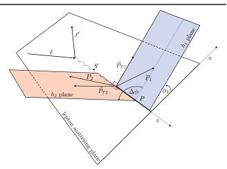
FIG. 1. The SIDIS kinematics of back-to-back dihadron production in the center-of-mass frame. The *x*-*z* plane is defined by the incoming and outgoing lepton with positive *z* in the direction of the virtual photon.  $\phi_1$  and  $\phi_2$  are defined from the scattering plane to  $P_1$  and  $P_2$  in an anticlockwise direction.
