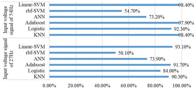
Figure 8. Fault detection accuracy comparison if only DFT is applied to voltage signals.
