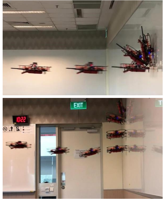
Fig. 6. Experimental demonstration of perching manoeuvre on vertical surfaces: Perching (top) and Release (bottom).
