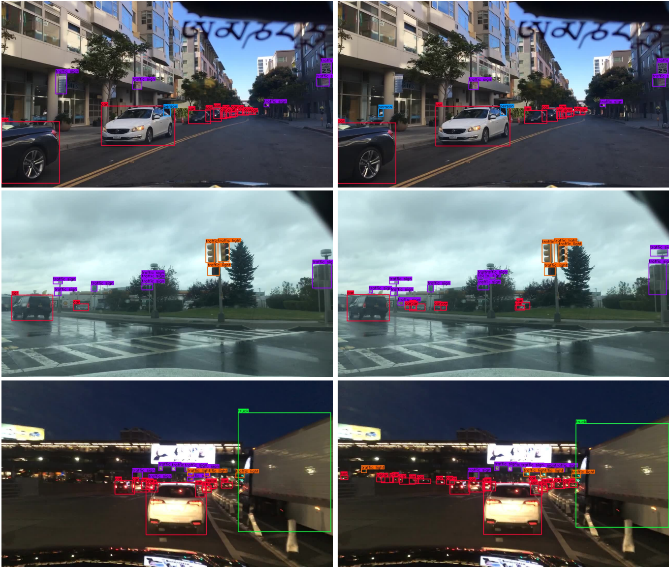
Fig. 9. Detection results of YOLOv3 and SA-YOLOv3 on BDD test set. The first column elaborates detection results of YOLOv3, while the second column demonstrates detection results of SA-YOLOv3.
