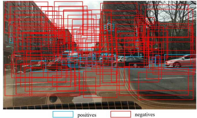
Fig. 1. The extreme positive-negative imbalance in one-stage detector. Postive sample is labeled by blue line, while bounding box with red line presents negative example.
