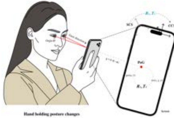
Fig. 1. The gaze estimation task involves predicting either a) a point of gaze (PoG) as a coordinate point on a screen (called 2D gaze) or b) a gaze direction in a 3D space (called 3D gaze) [31].
