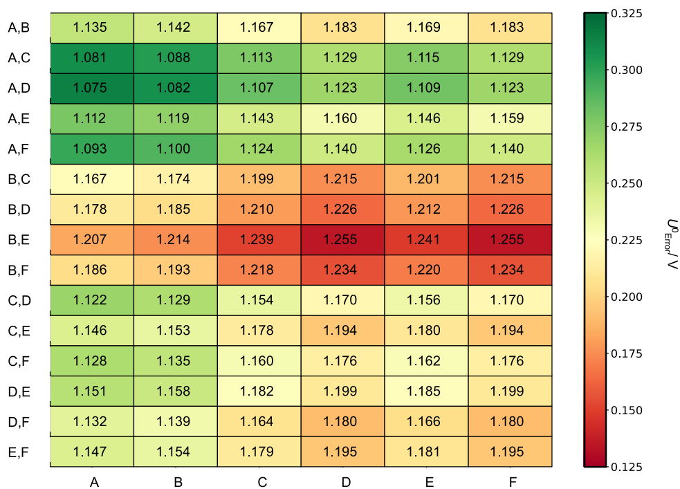
Figure 8. Redox potentials, U^0_{\text{Red}} vs SHE, for all cation rearrangements for K_x[\text{PW}_{11}\text{Co}(\text{H}_2\text{O})\text{O}_{39}]^{4-x} ; x = 4 or 5 , obtained using the PBE/TZP methodology. Gibbs free energies for all cation arrangements were computed using the zero-point energies and entropic components obtained from GGA—vibrational frequencies for A and A,D isomers. Experimental potentials were obtained from Co(III/II). 23,24
