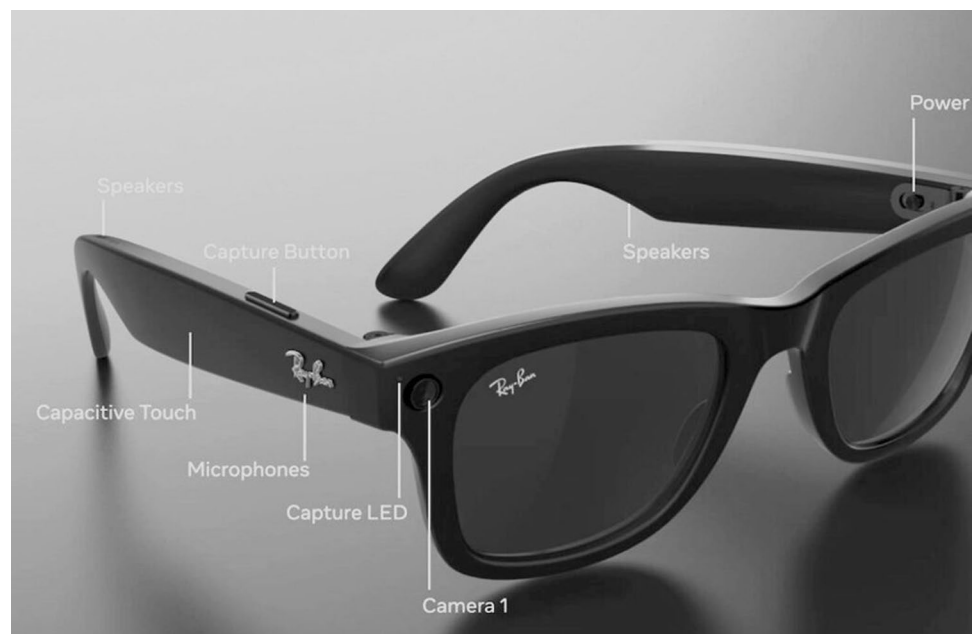
Fig. 1 Components of the Ray-Ban stories, camera, speakers, buttons, LED & microphones
