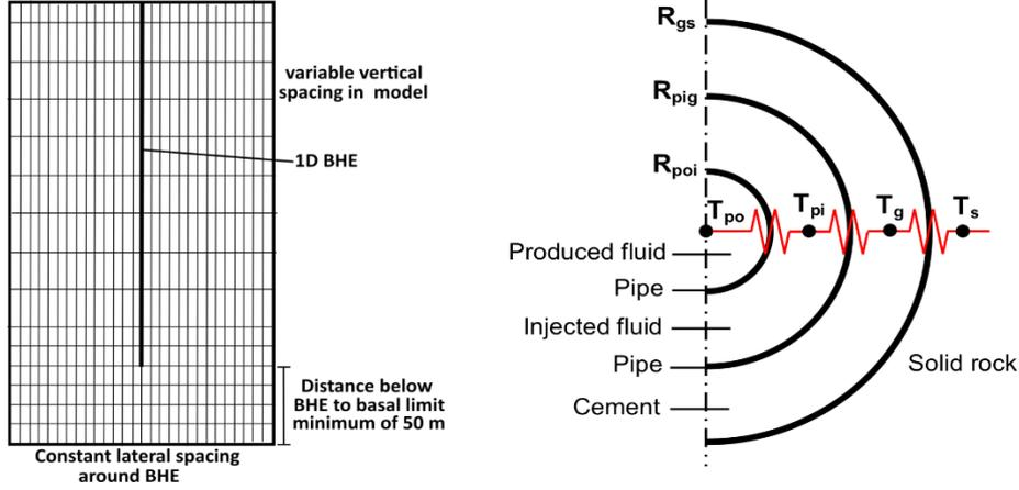
**Figure 4: Mesh discretization (left) and thermal resistances of casing materials, analogous to electrical resistances (right).**
