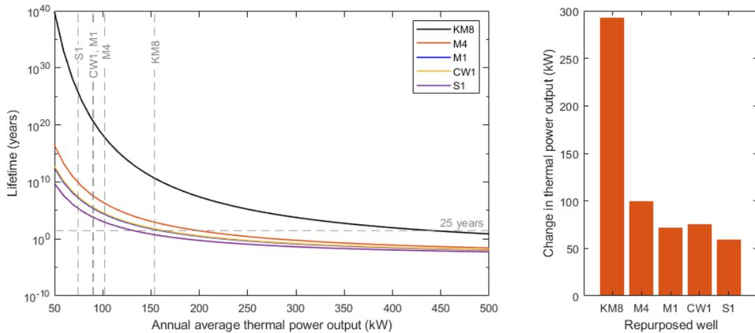
**Figure 9: Exponential relationship between the lifetime of deep borehole heat exchanger and average thermal power output, after Westaway (2018) (left), and the change in thermal power extraction required to obtain the maximum heat potential while maintaining a 25-year lifetime (right).**
