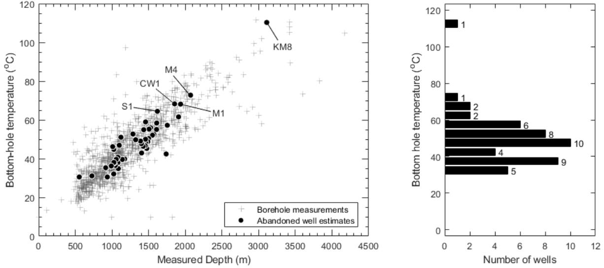
**Figure 3: Borehole measurement data from Burley (1984) and Rollins (1987) used to estimate bottom-hole temperatures of abandoned vertical hydrocarbon wells in the UK. KM8 = Kirby Misperton 8, M1 = Malton 1, M4 = Malton 4, CW1 = Crosby Warren 1 and S1 = Stainton A1.**
