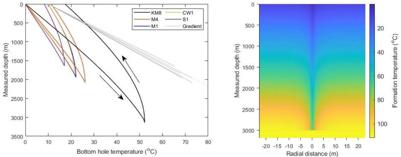
**Figure 6: Preliminary spatial temperature variations in DBHEs for the inlet annulus and outlet pipe along borehole depths (left) and the six-month radial thermal drawdown effect in the modelled KM-8 surrounding formations (right).**
