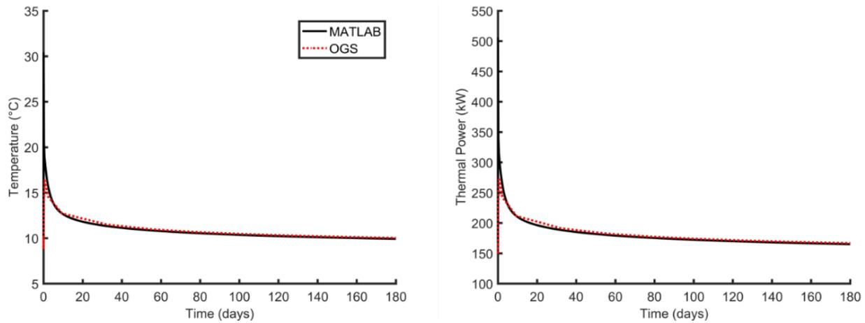
**Figure 5: Software comparison for outlet temperatures (left) and thermal power (right) of Crosby Warren-1 well. A 0°C inlet temperature is set to define the maximum achievable thermal power. All other parameters are listed in Tables 1 and 2.**
