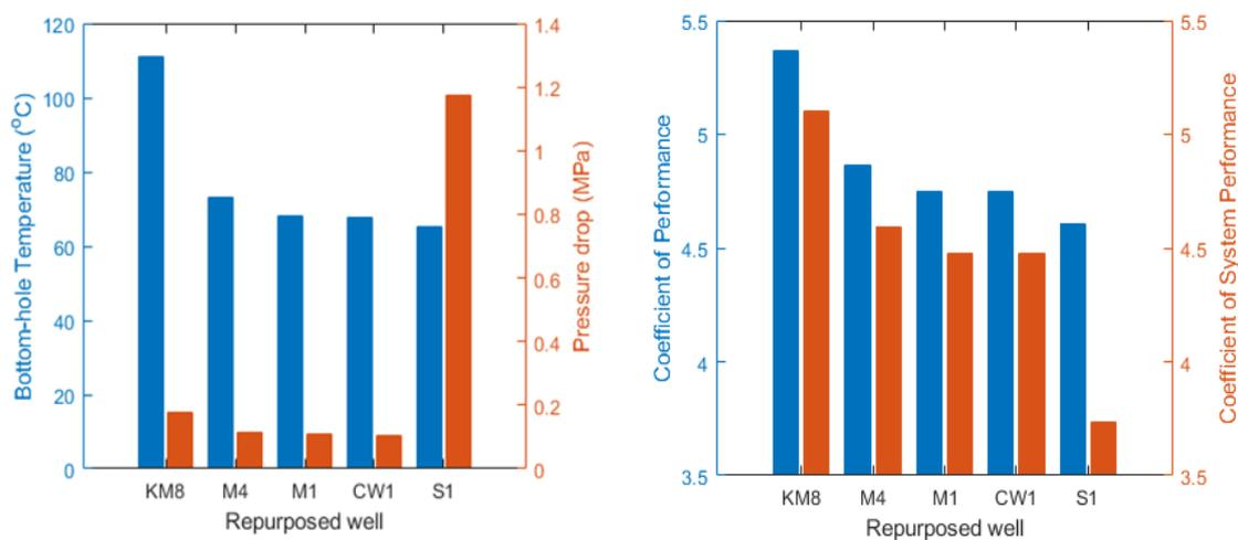
**Figure 8: Initial bottom hole temperatures and pressure drop after six months for candidate wells (left). Coefficient of Performance (COP) and Coefficient of System Performance (CSP) after six months of operating repurposed wells (right).**
