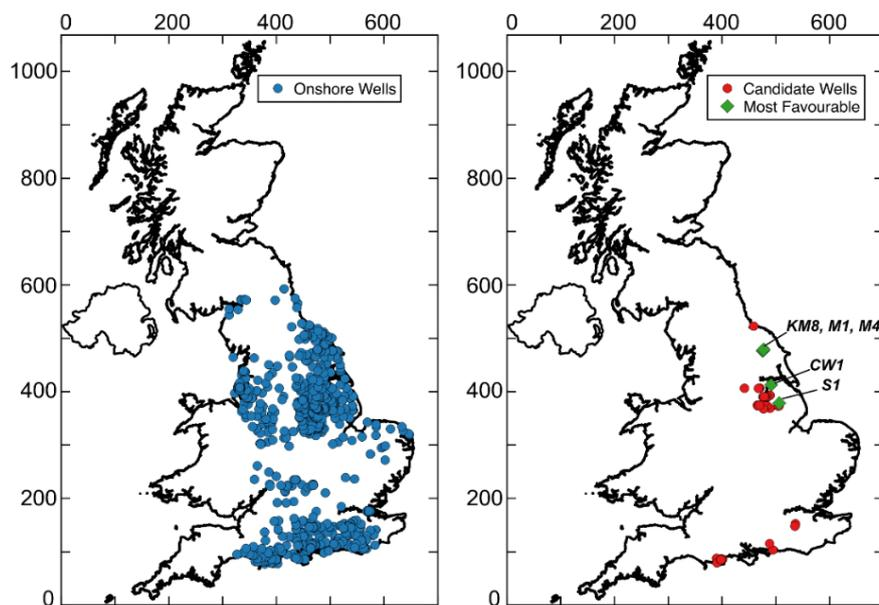
**Figure 2: Onshore hydrocarbon wells in the UK (left). Candidate and most favourable hydrocarbon wells for repurposing as DBHEs (right), using bottom-hole temperature for an initial metric of favourability. British National Grid coordinates (north and east) are in 100 km intervals. © Crown copyright and database rights 2022 Ordnance Survey (100025252).**
