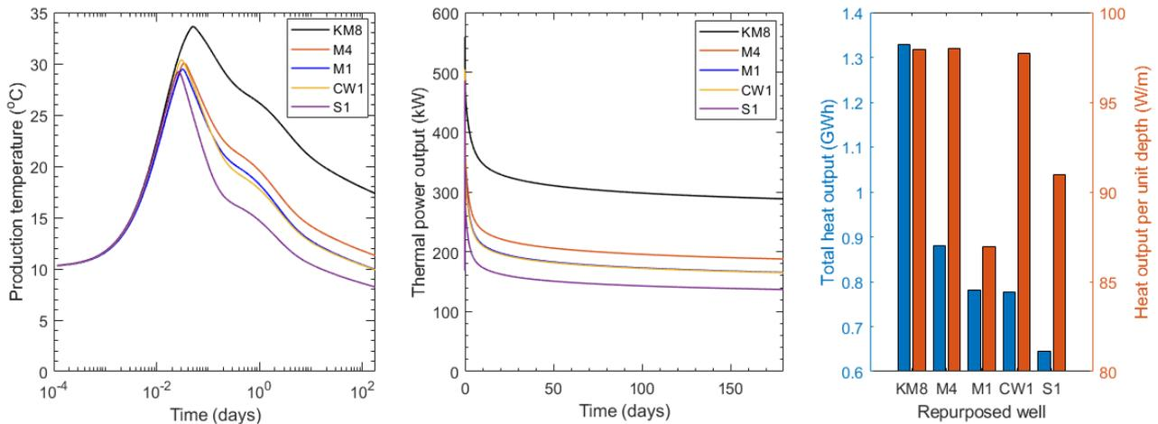
**Figure 7: Temporal variations in deep borehole heat exchanger outputs over a six-month heating season for temperature (left) and thermal power (middle). Cumulative heat supplied per well and per unit depth for each repurposed well (right).**
