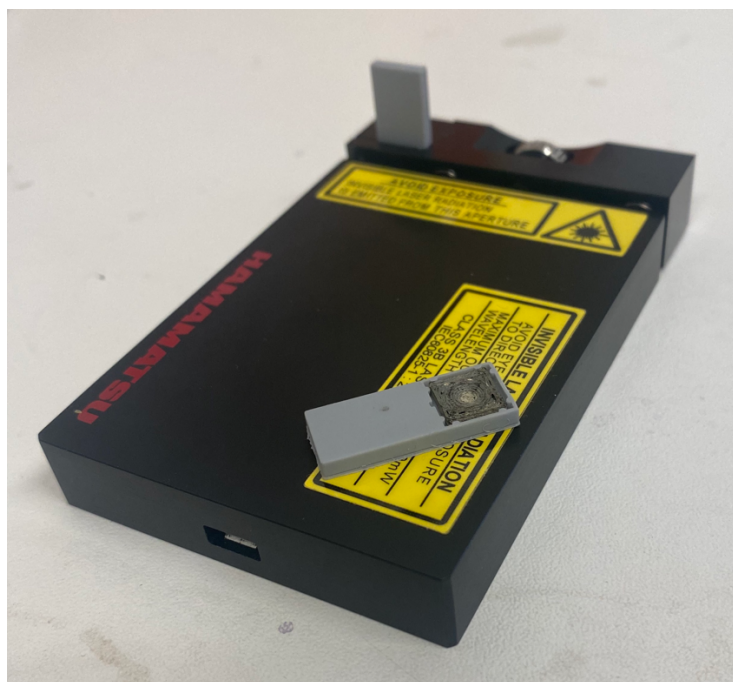
Figure S11: Ag/PP4% test strip with a drop of paraquat 100 \mu\text{M} to be used as SERS sensors using a portable Raman spectrometer.
