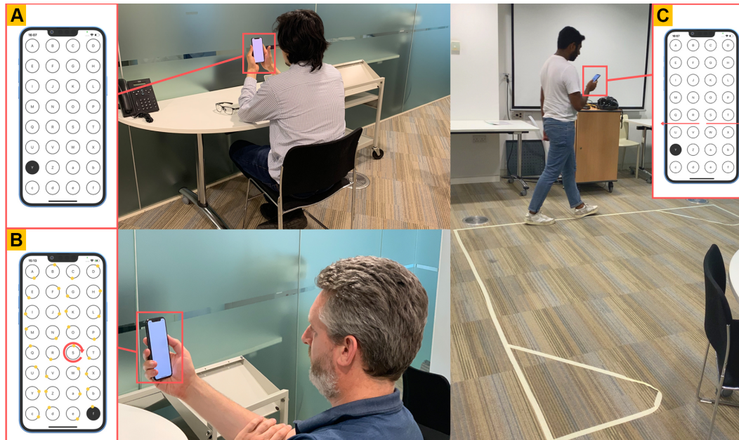
Figure 1: We evaluate the performance of the three widely used gaze-based interaction methods: Dwell time (A), Pursuits (B) and Gaze gestures (C), for target selections on handheld mobile devices while sitting (left) and while walking (right). All participants performed all selections using the three different techniques while sitting and while walking. The red arrow in (B) illustrates the direction in which a yellow dot stimuli was rotating around a selectable target. The red arrows in (C) indicate the directions in which the user could perform a gaze gesture. All arrows are for illustration and were not shown to participants.
