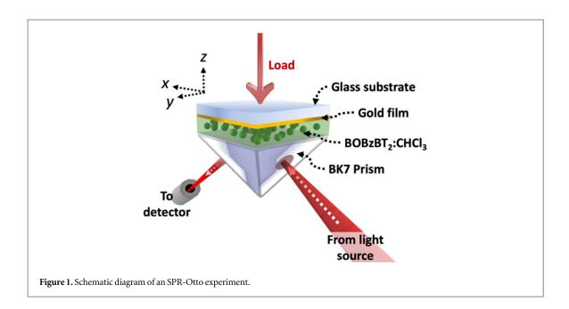
placing a 5 grams iron block on top of the back of Au-coated glass substrate and leaving it for 5 min to allow the excess deionized water to ooze out of the layer.
